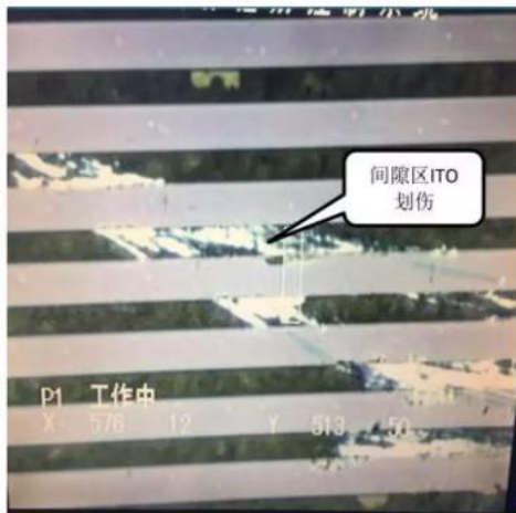
ITO scratches cause electrical shorts between phases
